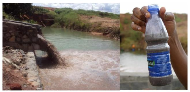
6 EFFLUENT FROM THE LUILU PLANT AND WATER SAMPLE TAKEN FROM THIS EFFLUENT.
